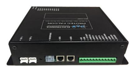
The Protec Falcon PFIQ is a programmable handheld siren and light controller, ideally suited for undercover and police management vehicles. The hand held controller can quickly be concealed if the situation requires it. The system is available in 12 and 24 volts and is easily installed by a trained technician.
